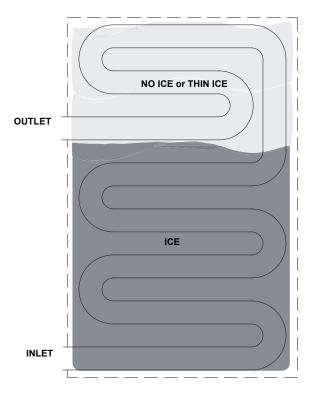
Figure 7-3. Extremely Thin Ice Formation at Evaporator Outlet
